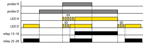
PUMP DOWN, ON DELAY (Function 6)
